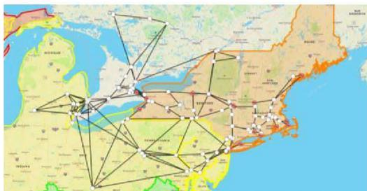
Fig.4. NPCC 140 Bus System Single-line Diagram
