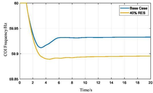
Fig.6. System frequency response with 40% renewable energy source penetration
