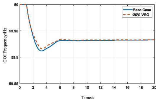
Fig. 8. System frequency response with 20% VSG controlled renewable energy source penetration
