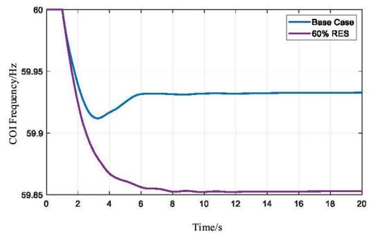
Fig.7. System frequency response with 60% renewable energy source penetration
