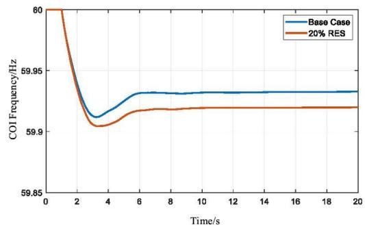
Fig.5. System frequency response with 20% renewable energy source penetration
