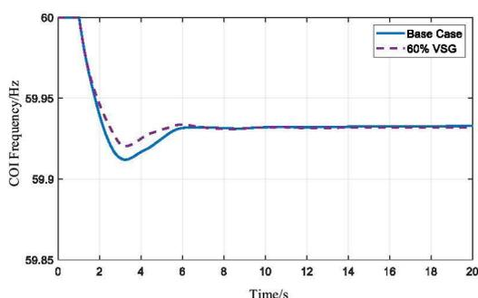
Fig. 10. System frequency response with 60% VSG controlled renewable energy source penetration
