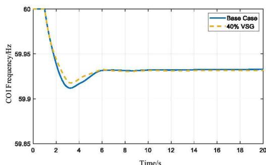
Fig. 9. System frequency response with 40% VSG controlled renewable energy source penetration
